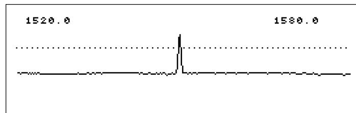
PRBS modulation graph showing raised noise floor.
